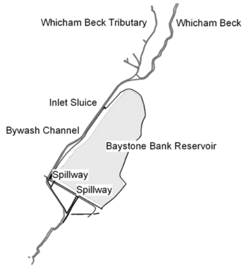
Figure 1. Hydraulic arrangement of Baystone Bank Reservoir
